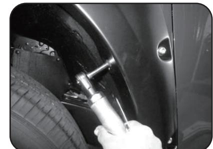
Start Screw (SW1-0036) through the three lower rear holes in flare and into factory holes in rear of wheel well.
