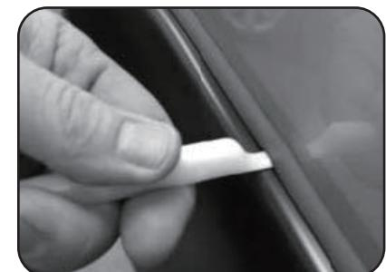
Using flat end of supplied Edge Trim Tool (ET1-0001), seat edge trim against flare by inserting straight end between edge trim and flare at one end. Next, slide around entire edge to the other end.
