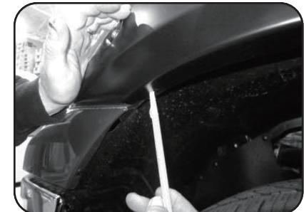
Hold front of the flare firmly on the fender. Mark three Clip (CL1-0005) locations using the holes in the flare as a guide.
