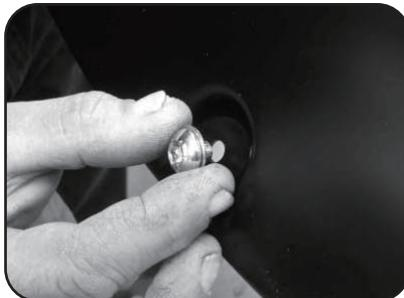
Put a Washer (WA1-0012) on each Bolt (SW1-0059). Put each Bolt through a pocket hole in the flare, bolt head on the outside.
