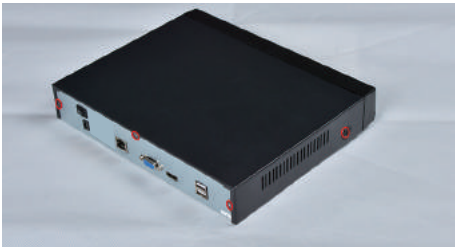
Remove the top two screws
