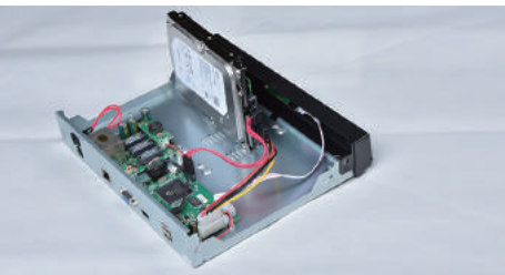
Connect data wire and power wire as shown
