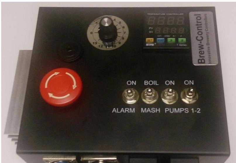
A red mushroom button at the bottom left that serves as an on/on switch as well as a panic stop button. Twist the mushroom button to the right to turn on main power and push the mushroom button in to turn off main power.
