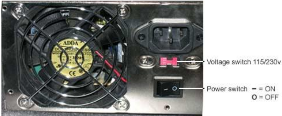
Figure below shows typical cable connection found on the power supply
