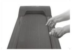
Pull up the running belt tightly. Then put the silicone oil to running board. Then start the machine to running 3 minutes without loading. It is better to maintain like this every 30 working hours of the machine. This can save the lifetime of parts.
