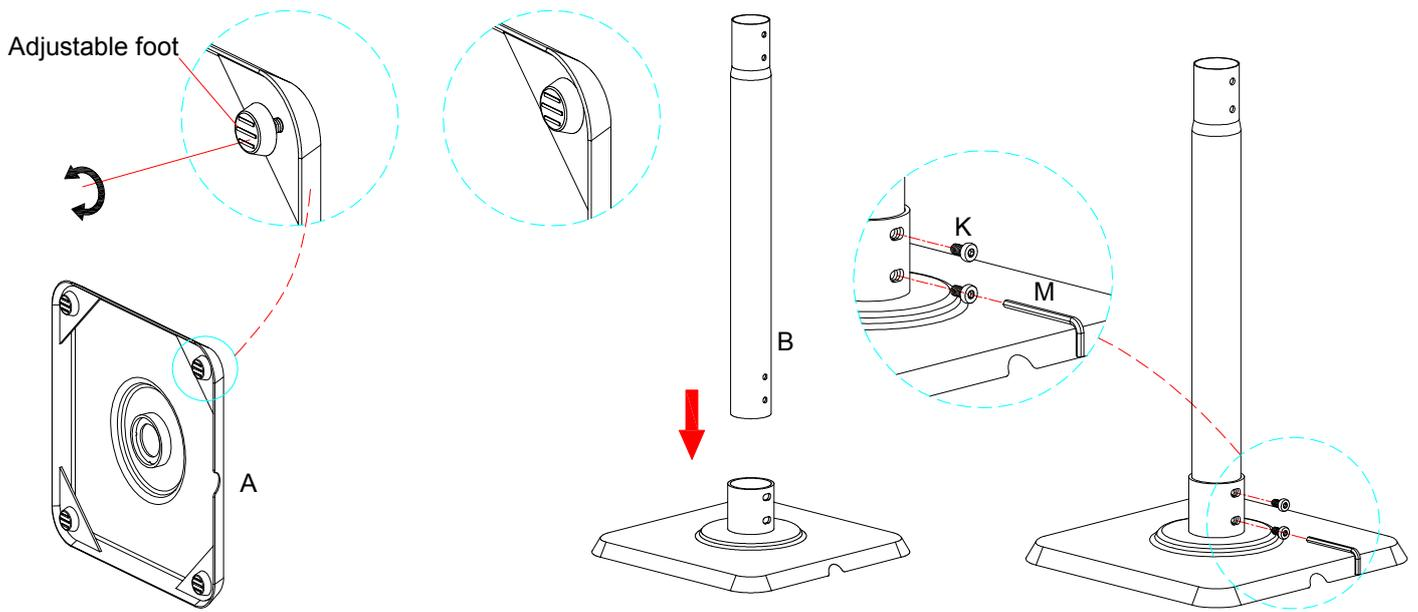
**Step 2** Insert upper tube (C) into bottom tube (B) and use Allen key (M) to fasten bolt (K).
