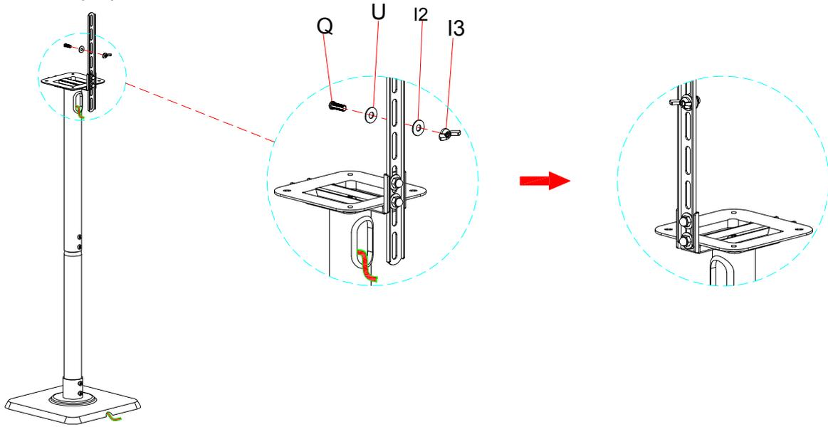
Place speaker on stand with key hole bolt (Q) inserted in the key hole, then tighten the nut (I3) and plug the wires.
