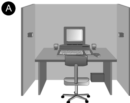
Rear satellites mounted on walls behind you
