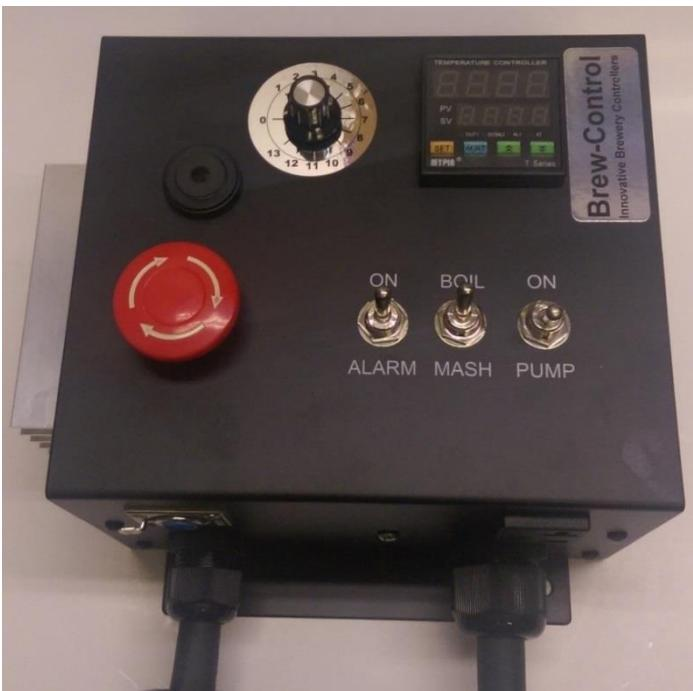
A red mushroom button at the bottom left that serves as an on/on switch as well as a panic stop button. Twist the mushroom button to the right to turn on main power and push the mushroom button in to turn off main power.
