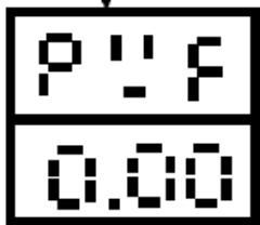
**This is the offset value used to calibrate your thermocouple.**
