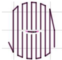
Figure 2.39: Support infill pattern: Rectilinear
