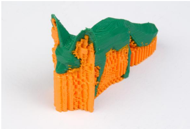
Figure 2.17: An example of an object printed with support material.
