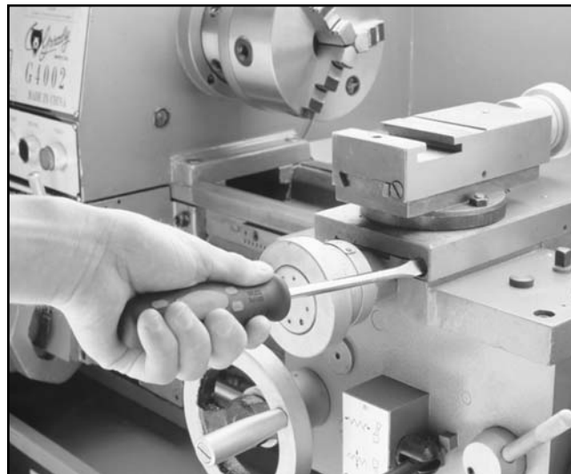
Figure 25. Adjusting the cross-slide gib.
