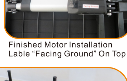
Finished Motor Installation Label "Facing Ground" On Top
