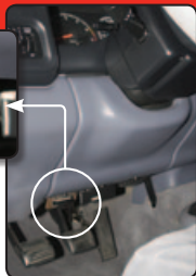
Typical OBDII Connector location
