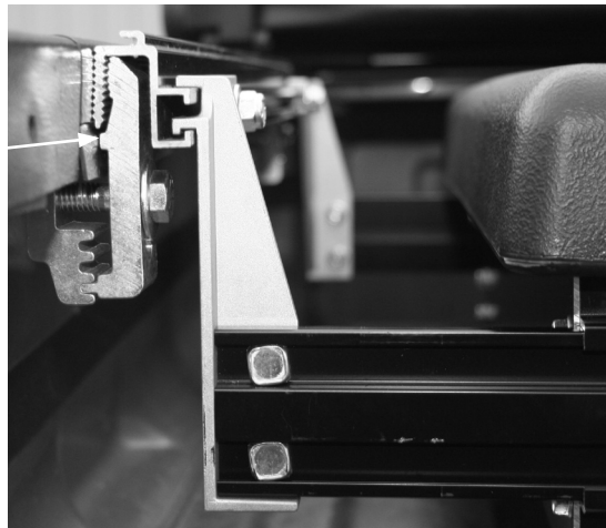
Install clamps towards end of mounting rail
