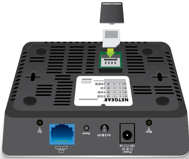
Figure 2. Overview of installing the micro SIM card
