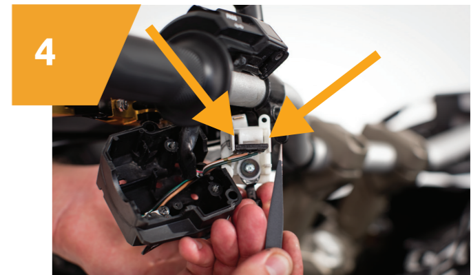
4 Insert supplied foams into turn signal switch. More info
