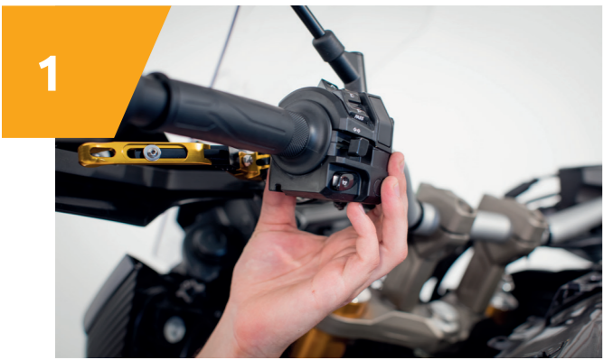
1 Locate the cable coming from left handlebar switch and find an accessible spot.
