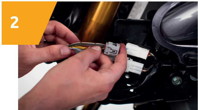
2 Remove main insulation, locate and cut 3 wires (left, right and flasher signal wire), and crimp red bullet connectors. Then locate power supply* (12 V and GND).
