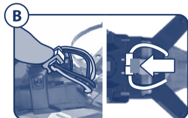
Align forward facing edge of connectors against short tabs before snapping into locked position against connector's tab.
