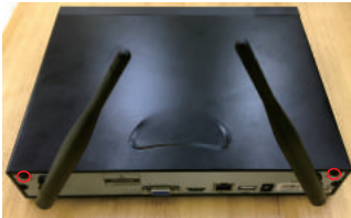
Remove the cover from the unit, and remove the top two screws
