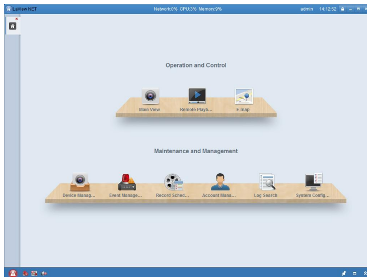
Figure 3-5 LaView NET Control Panel
