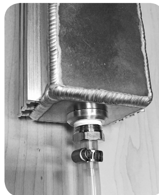
Tubing attached to bottom of Overflow tank
