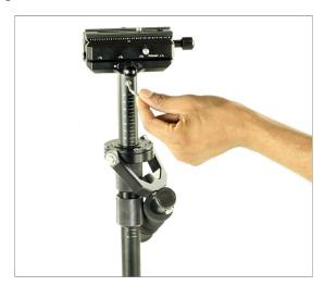
• Attach the quick release plate to the camera base. Slide the release lever to insert the camera set up into quick release adapter. Return the lever to its original locked position.
