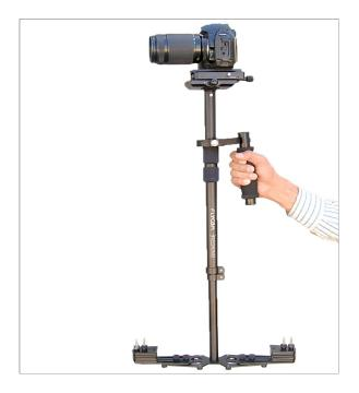
When testing for correct horizontal balance you need to make sure that you pick up your Stabilizer from a flat surface (a table for example) and that you let the Stabilizer hang freely as you hold it. If the Stabilizer is balanced correctly, on it's horizontal axis, then it will be level with the central post in a virtually perfect vertical position.
