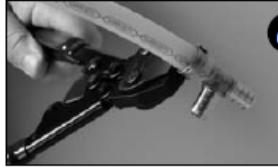
4 Position Clamp Tool jaws over raised tab of clamp ring and squeeze.
