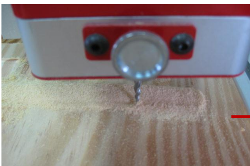
When wood texture is paralleled to X axis, wood chips would accumulate on the cutter.
