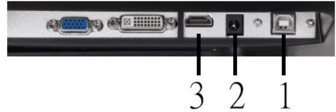
Image 2-1: Connection (1:USB port; 2 :Power jack; 3 :HDMI port)
