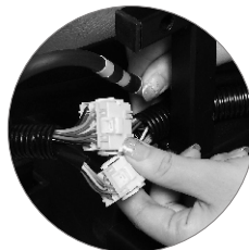
Connect Air Hose And Leg Rest Wire Connection To The Main Body Carefully And Complete
