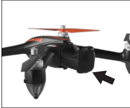
SLIDE BATTERY IN COMPARTMENT
