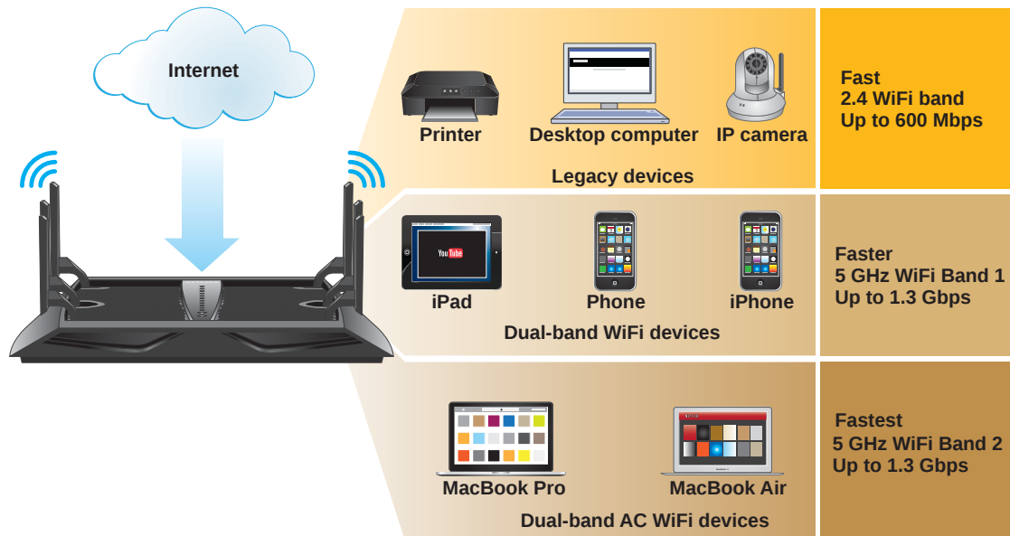
Figure 9. Load balancing in a tri-band WiFi network
