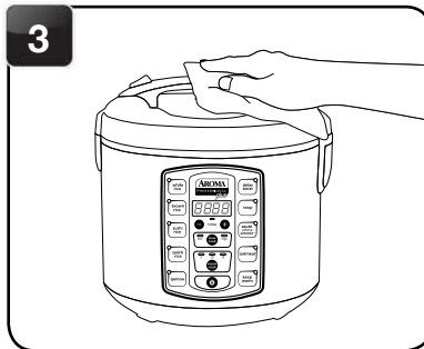
3 Wipe rice cooker body clean with a damp cloth and thoroughly dry rice cooker body and all accessories.
