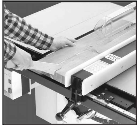
Figure 51. Typical ripping operation.
