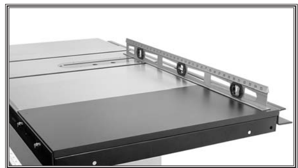
Figure 22. Adjusting Model W1819 extension table flush with wing and table.
