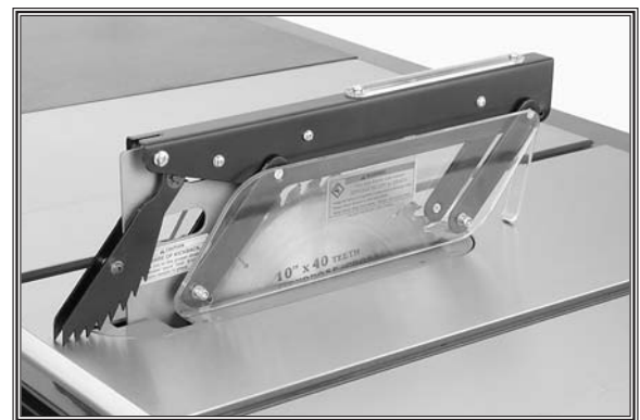
Figure 31. Blade guard installed.
