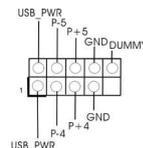
Besides two default USB 2.0 ports on the I/O panel, there are three USB 2.0 headers on this motherboard. Each USB 2.0 header can support two USB 2.0 ports.
