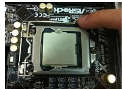
Step 3-2. Press down the load lever, and secure it with the load plate tab under the retention tab. The protection cover will automatically come off by itself.
