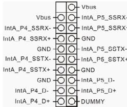
Besides four default USB 3.0 ports on the I/O panel, there is one USB 3.0 header on this motherboard. This USB 3.0 header can support two USB 3.0 ports.
