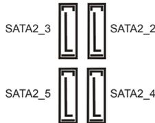
These four Serial ATA2 (SATA2) connectors support SATA data cables for internal storage devices. The current SATA2 interface allows up to 3.0 Gb/s data transfer rate.
