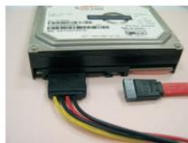
**Step 2** Unplug SATA 15-pin power cable connector (Black) from SATA / SATA2 / SATA3 HDD side.
