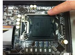
Step 1-2. Keep the lever positioned at about 135 degrees in order to flip up the load plate.
