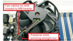
Step 3. Align fasteners with the motherboard through-holes.
