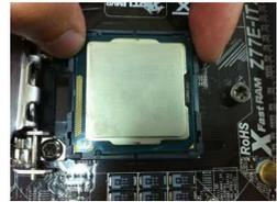
Step 2-4. Verify that the CPU is within the socket and properly mated to the orientation keys.
