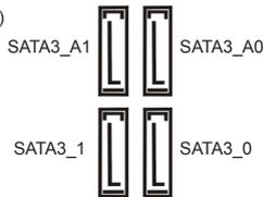
These four Serial ATA3 (SATA3) connectors support SATA data cables for internal storage devices. The current SATA3 interface allows up to 6.0 Gb/s data transfer rate. If the eSATA3 port on the rear I/O has been connected, the internal SATA3\_A1 will not function.
