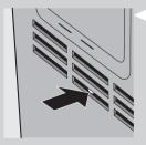
7 Put filter 1 (HEPA filter) back into the appliance.
