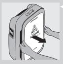
1 Place your fingers in the recesses of the side panels and gently pull the top part of the front panel towards you. Then lift the hook at the bottom of the panel out of the bottom of the appliance.
