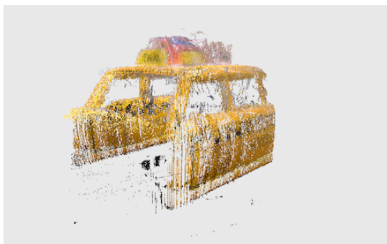
Example of center out cropping (all points removed in a radius of 31.6 mm from center)
