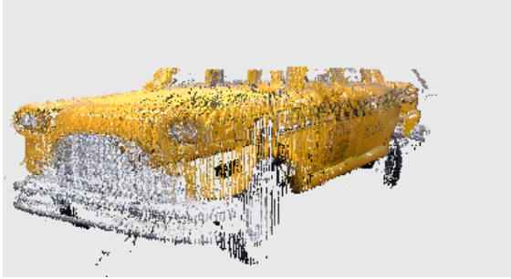
Example of top down cropping (all points removed above 38 mm from base)
