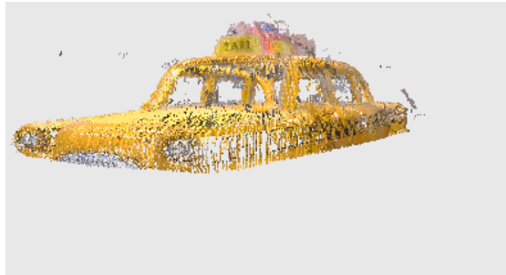
Example of bottom up cropping (all points removed below 24.7 mm from base)
