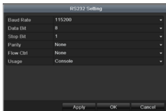
Figure 13. 7 RS232-Receive port Settings Interface
