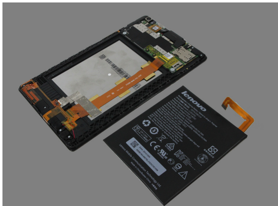
Figure 2-7. The removed battery pack
