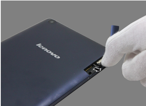
Figure 1-2. Removing the dual micro SIM card tray (Lenovo TAB 2 A8-50L/LC only)
