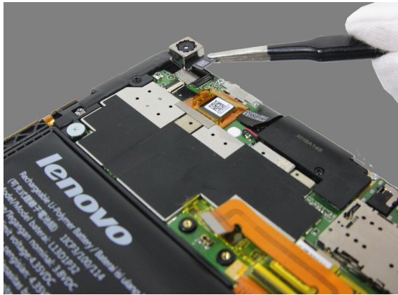
Figure 3-2. Removing the rear camera
