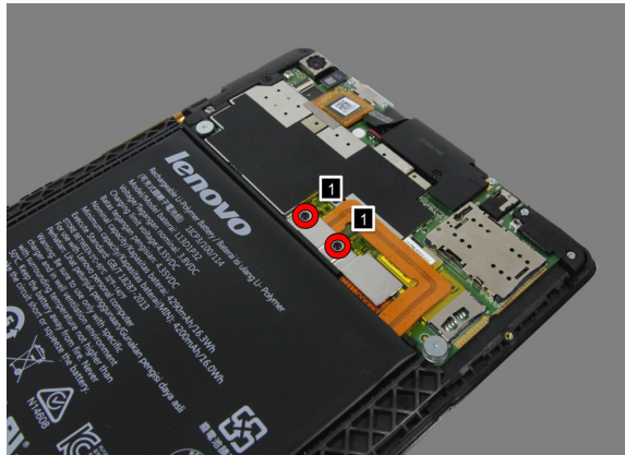
Figure 2-1. The screws on the metal piece for fixing the battery FPC
