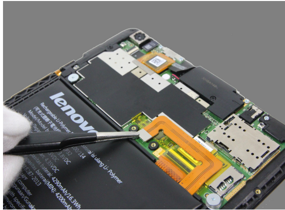
Figure 2-3. Disconnecting the battery FPC
