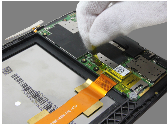
Figure 5-5. Removing the mylar on the main FPC (main board side)
