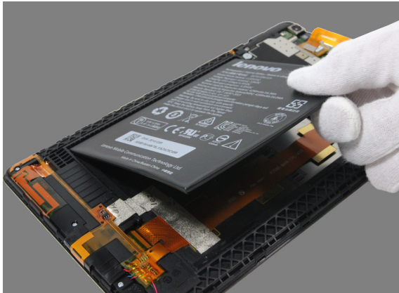
Figure 2-6. Removing the battery pack
