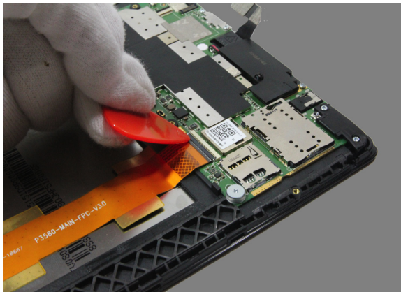
Figure 6-2. Unlocking the connector of the main FPC
