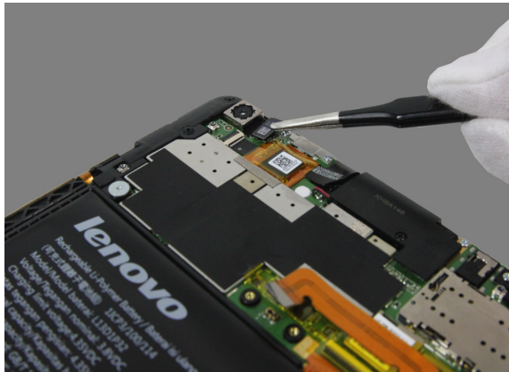
Figure 3-1. Detaching the connector of the rear camera FPC
