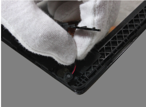
Figure 6-17. Detaching the microphone
