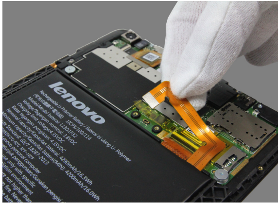
Figure 2-4. Detaching the battery FPC
