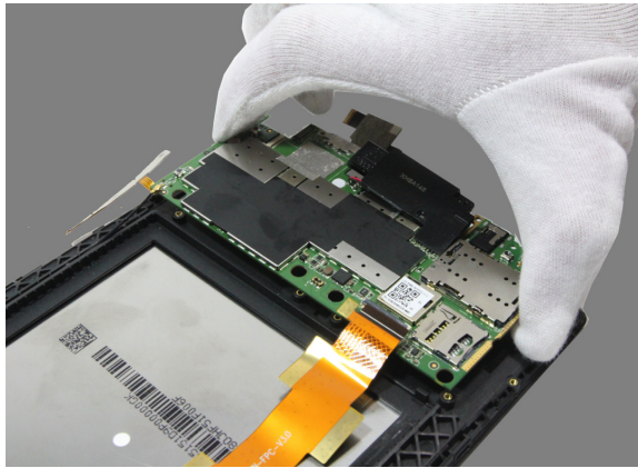
Figure 5-12. Removing the main board assembly
