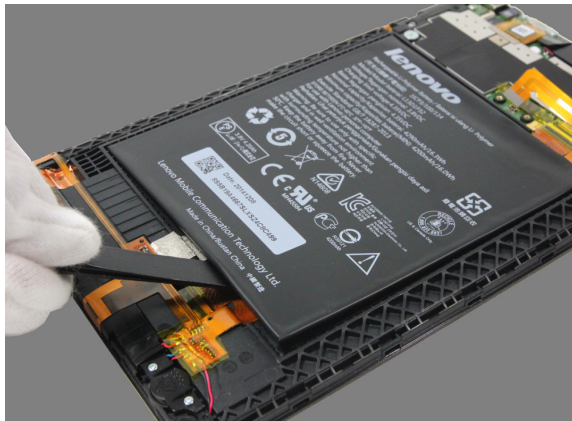
Figure 2-5. Detaching the battery pack
