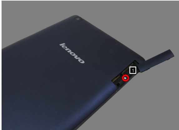
Figure 1-3. The screws on the rear cover
