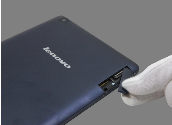
Figure 1-1. Opening the SD/SIM card cover
