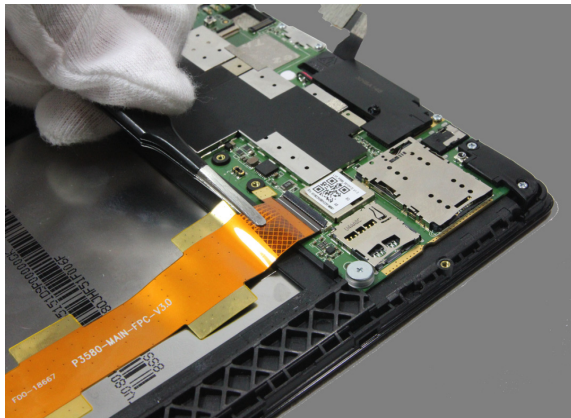
Figure 5-7. Pulling out the main FPC (from the main board side)
