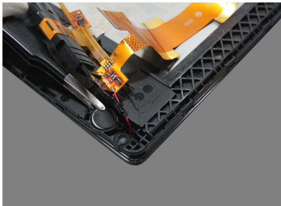
Figure 6-16. Detaching the vibrator
