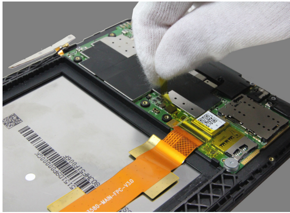
Figure 6-1. Removing the mylar on the main FPC (main board side)
