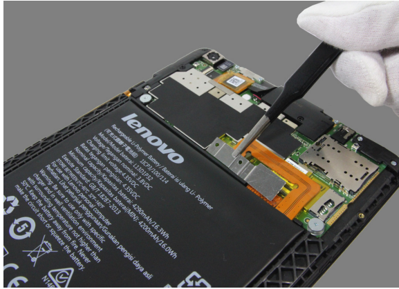
Figure 2-2. Removing the metal piece
