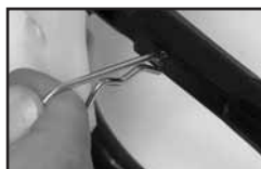
Figure 2 Line up holes
