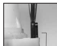
Guide edge facing away from pressure cylinder
